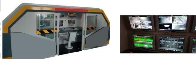
Figure 2. Cabin for monitoring the automatic operation of the MIKRUS system from the surface
