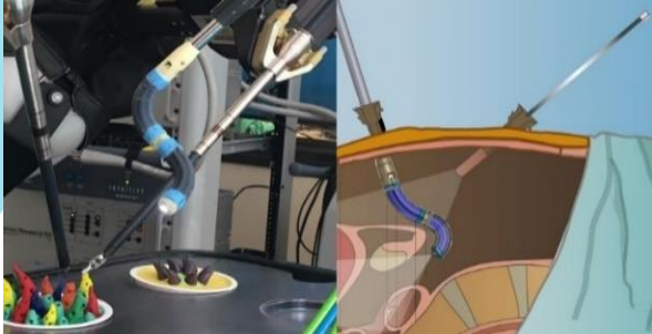
Figure 4: Soft Robot performing invasive surgery
